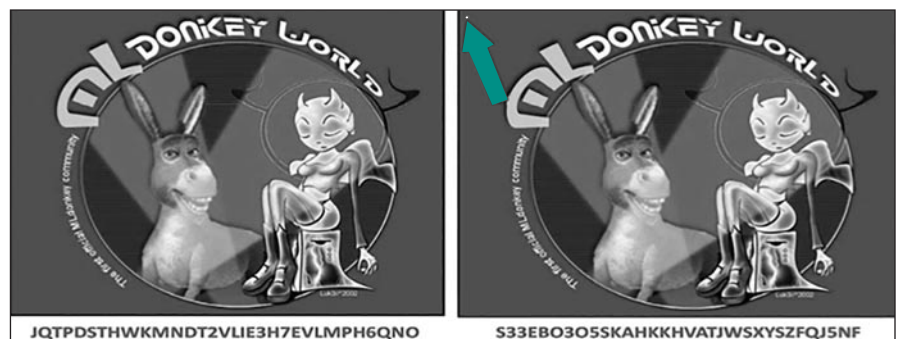
These two images differ by a single pixel (the green arrow is pointing to a tiny white dot in the right image), which is enough to change their SHA1 values (at the bottom of each image).
