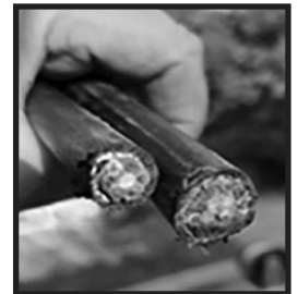
The inside of a communication cable.
